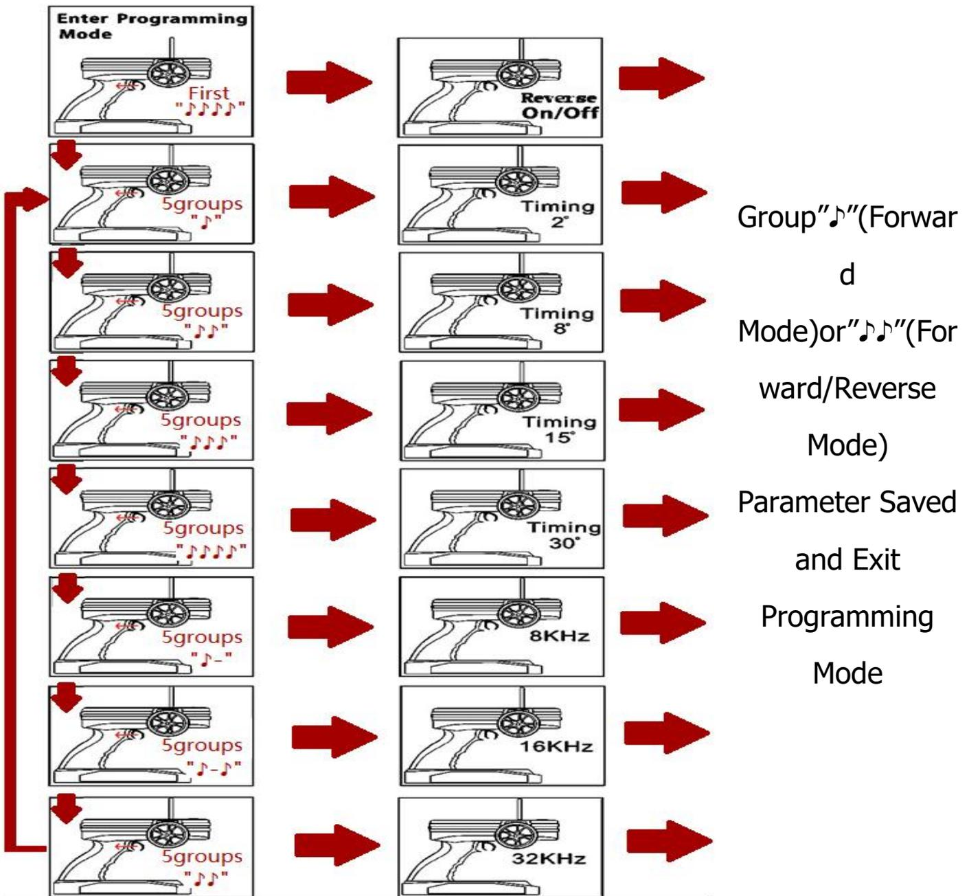
1. Move the stick of the transmitter to the full throttle position, and power on the receiver.
