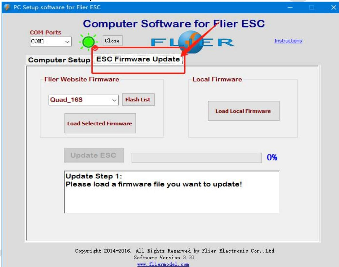
1. Disconnect all the connections to the ESC. Insert the USB cable into the USB port of the computer, and run the software. Please kindly notice whether the right port is selected.
